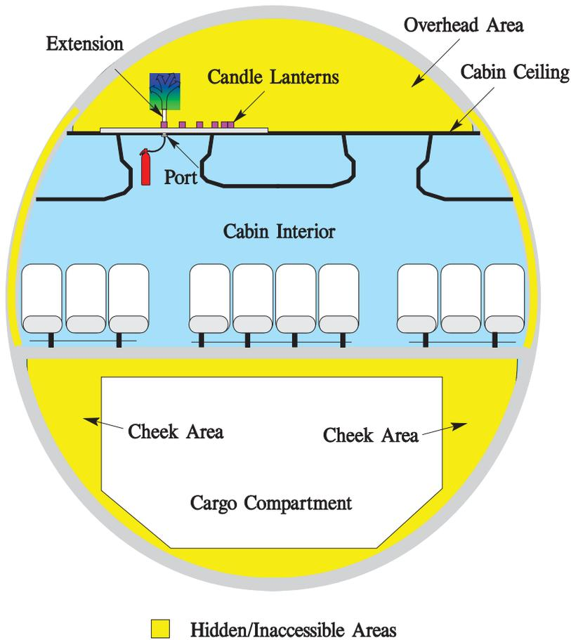
Figure 15. Candle Lanterns Located Directly Above Ceiling Panel
