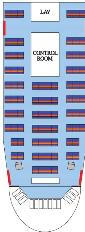
Figure 3. B-747SP Wide-Body Aircraft Test Section Schematic
