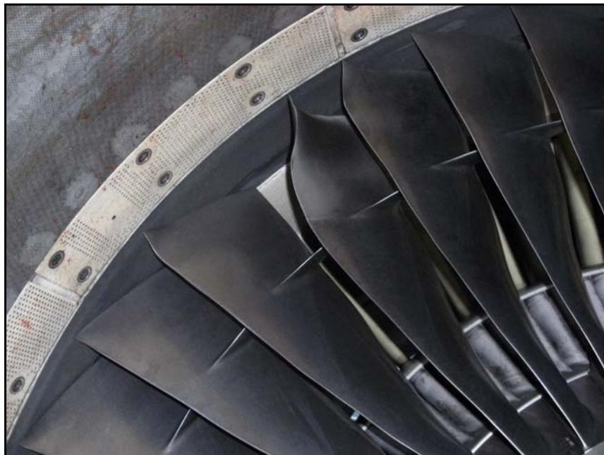
**Photo No. 1: No. 1 Engine Fan Blade Damage**
