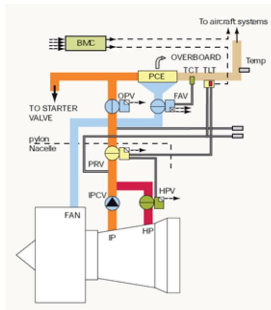
Figure1. General layout of the bleed air system
