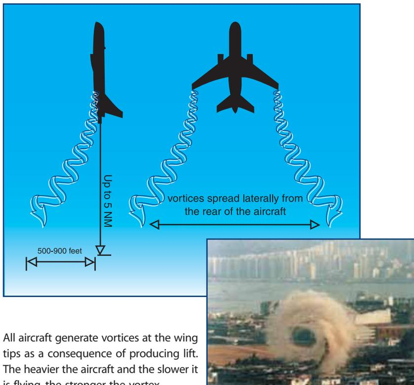
All aircraft generate vortices at the wing tips as a consequence of producing lift. The heavier the aircraft and the slower it is flying, the stronger the vortex.
