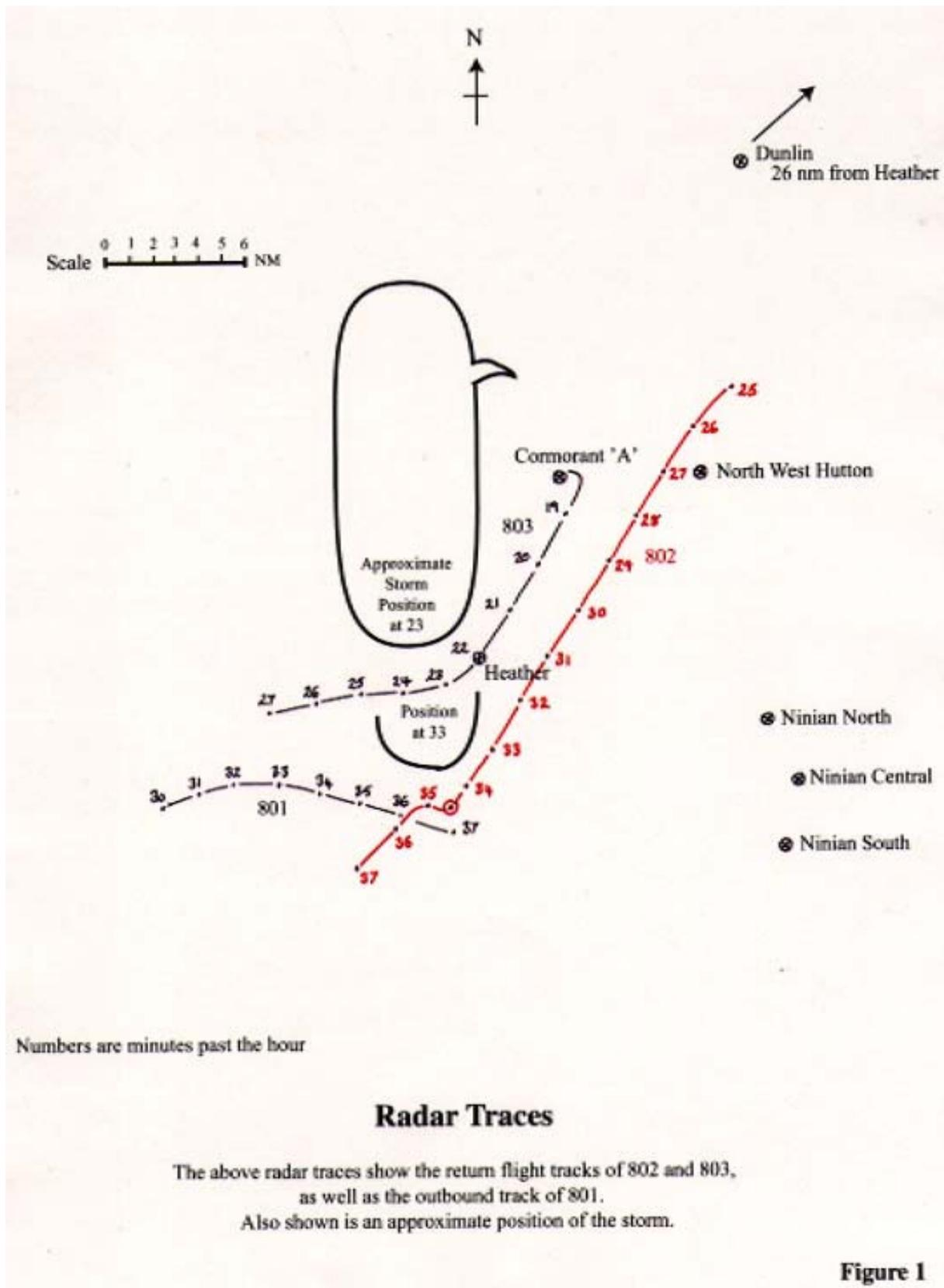
The departure of 802 was uneventful and the helicopter became established in the cruise at 130 kt IAS (160 kt ground speed) on a south-westerly heading at the assigned altitude of 1,000 feet. The autopilot was engaged, altitude hold was selected on the flight director and the crew had their hands and feet clear of the controls.
