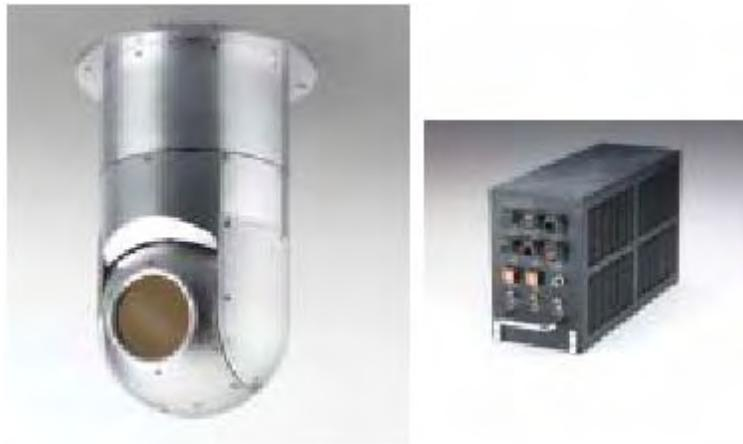
Figure 29. The LOAS Scan Head and Electronics [20]
