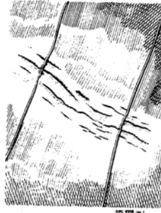
Tube Creasing Figure 315
