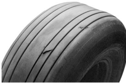
Cut Damage Figure 303
