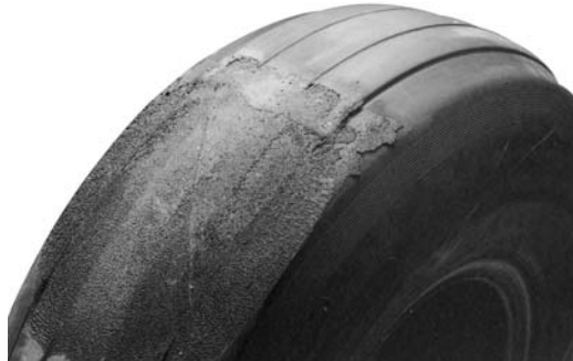
Wet Braking Flats Figure 305
