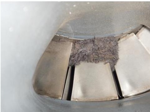
**Figure 1.** IGVs with material.
