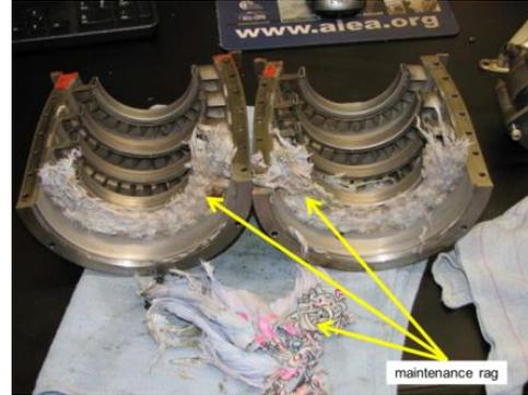
**Figure 4.** Compressor case halves removed.
