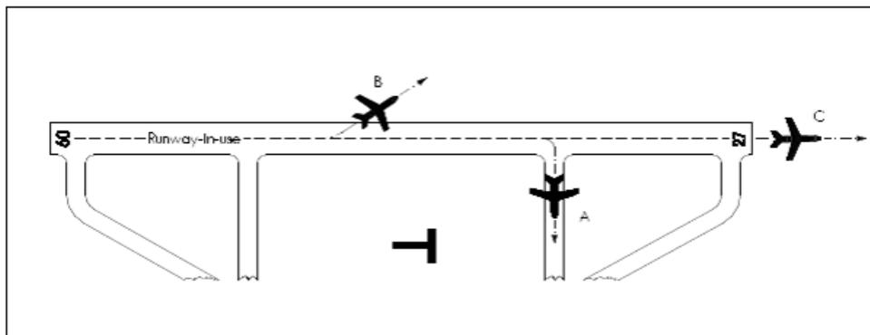
**Fig. 3:** Figure 9-3 shows the positions to be reached by a landing aircraft (A) or a departing aircraft (B or C) before an arriving aircraft may be cleared to cross the threshold of the runway-in-use, or a departing aircraft may be cleared to take off
