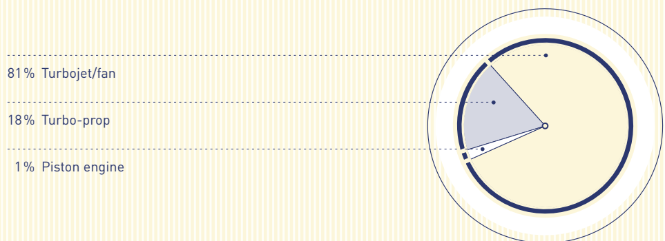
FIGURE 8 Public air transport fleet, distribution by type of propulsion, ICAO contracting states 1996 – 2005, aircraft mass greater than 9,000 kg MTOM
