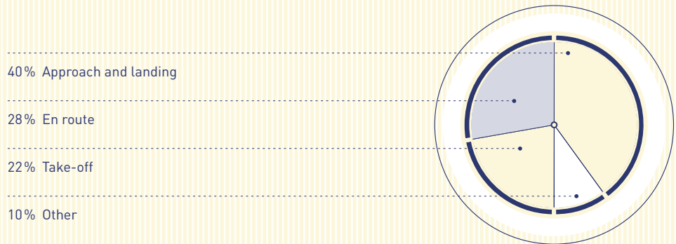
FIGURE 7 Distribution of fatal accidents over the phases of flight, world, public transport operations, 1997 – 2006, fixed wing aircraft over 2,250 kg MTOM
