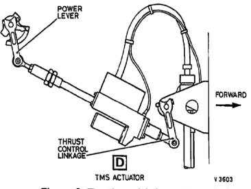
Figure 6: Throttle modulation system actuator
