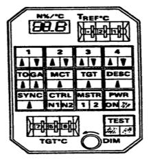
Figure 5: Control Display Unit (CDU)
