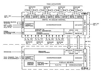
Figure 7: Block diagram of TMS
