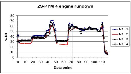
Figure 3: Graph of all-four-engine rundown
