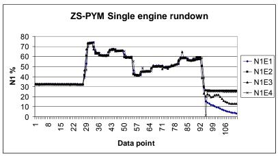
Figure 2: Graph of single-engine rundown
