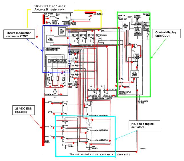
Figure 4: Wiring diagram of the TMS
