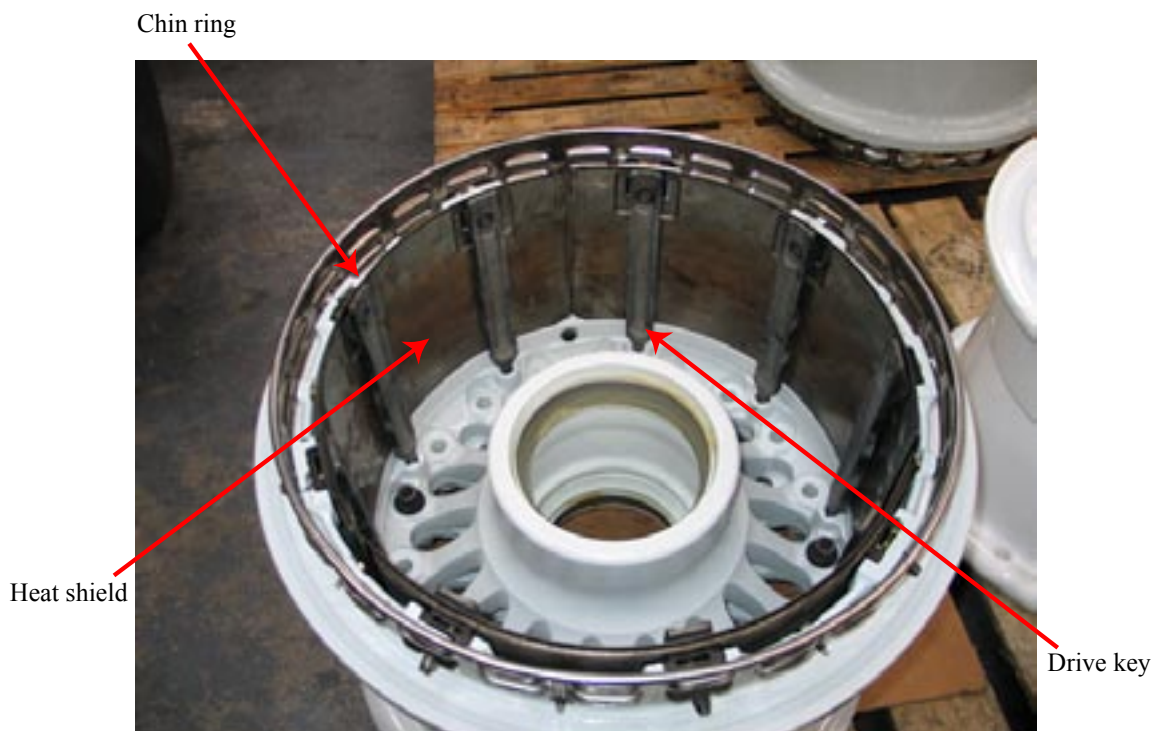
Figure 4 Construction of main wheel
