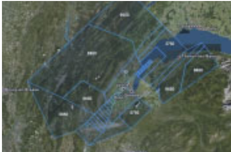
Birds Eye view of the current MSAW polygons in use at Geneva (altitude in feet)
