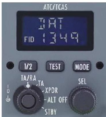
The Aircraft ID (also known as the Flight ID) is to be entered through the FMS or transponder control panel (depending upon aircraft equipment).
