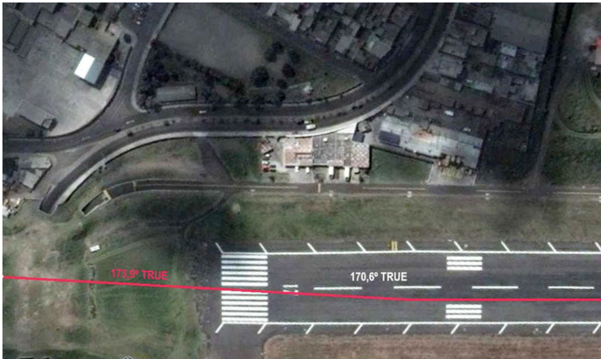
Figure 14. Final part of the aircraft's path obtained from FDR coordinate data adjusted to the point on the runway where the aircraft came to a stop. Photo property of Google Earth
