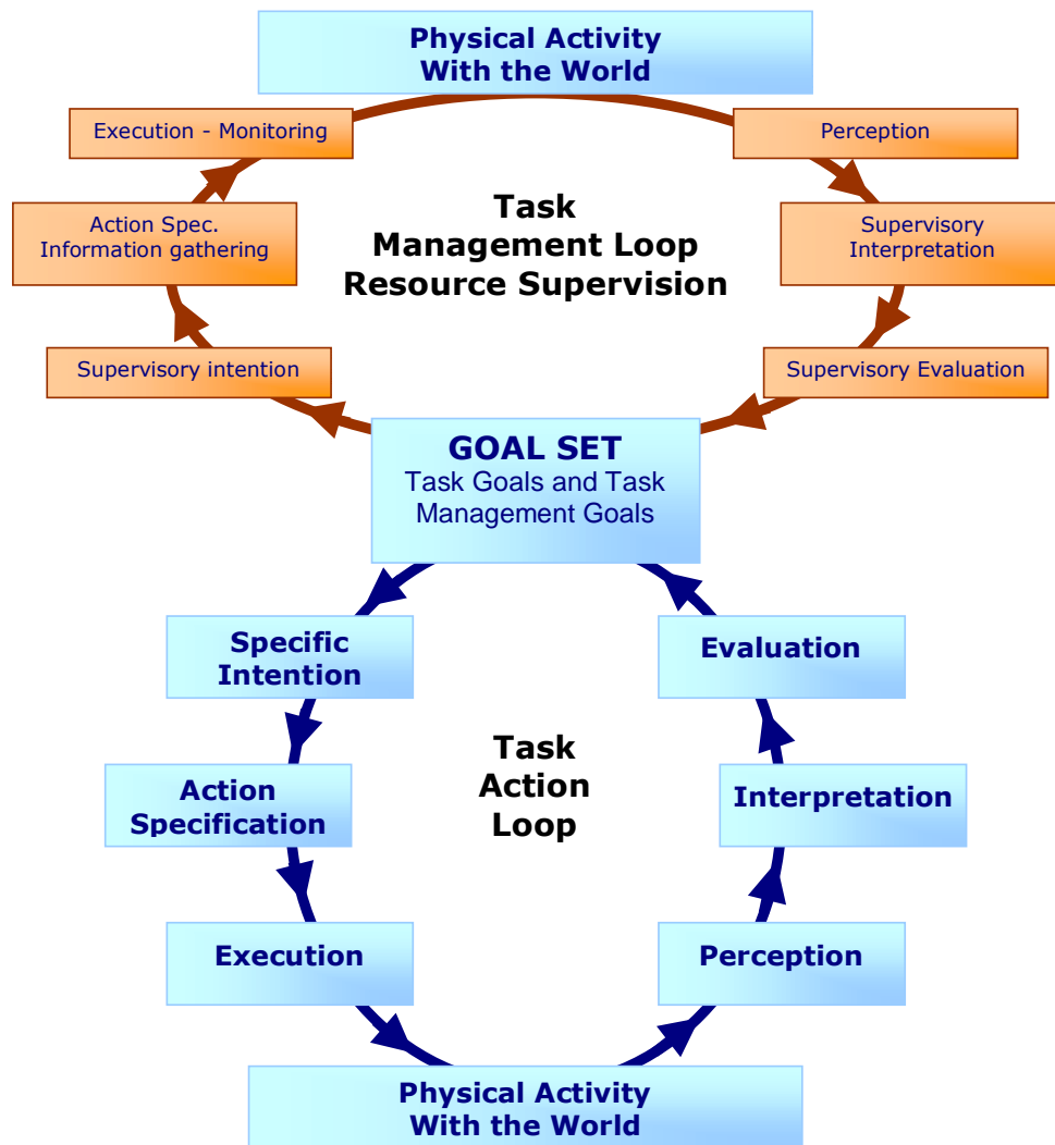
Figure 7: The Norman Model extended to include the Supervisory Loop (from [24])
