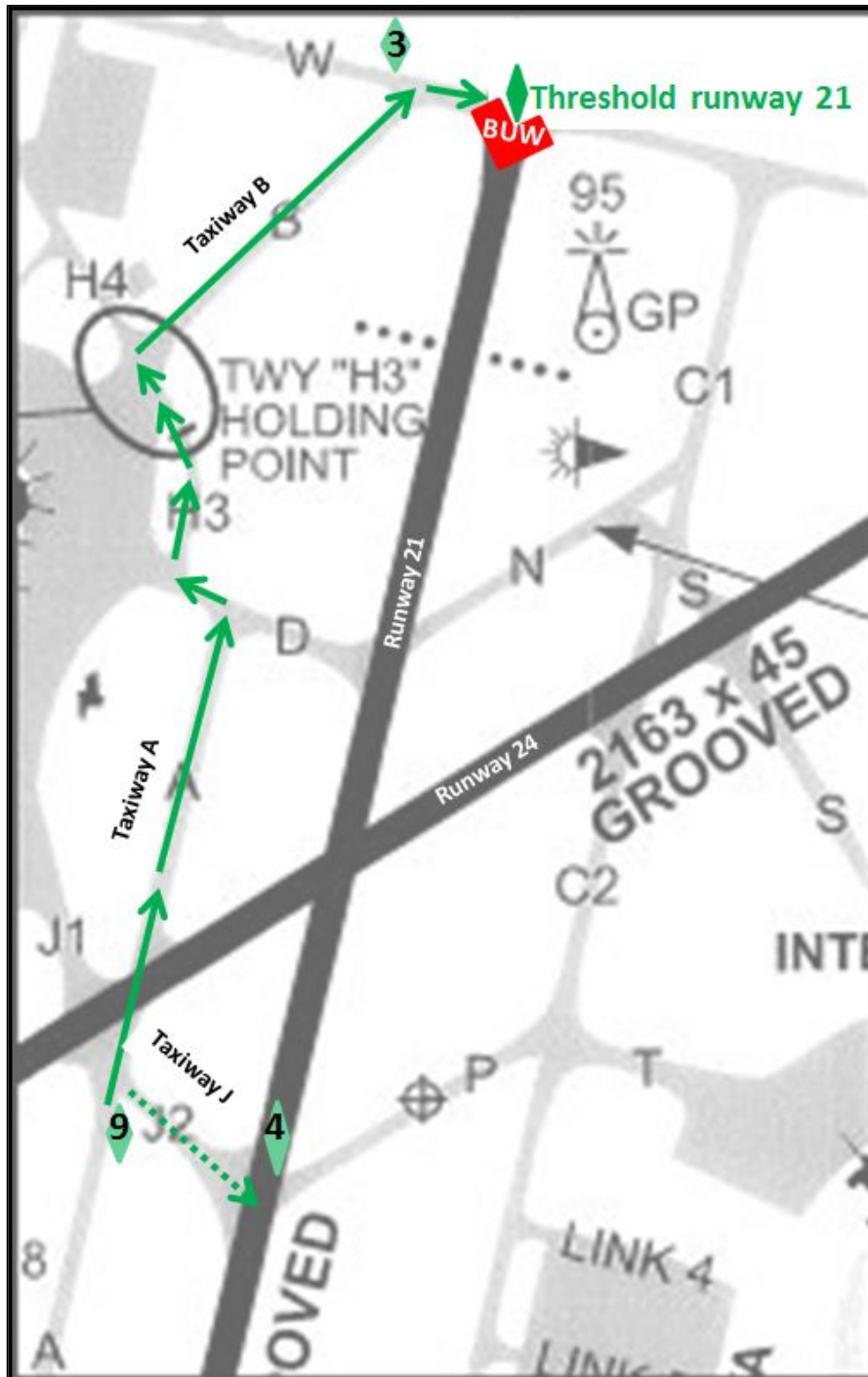
Figure 1: Location of safety vehicle positions (green diamonds), actual path of Safety 2 (dotted green line), path of Safety 2 as intended by ATC (solid green line) and location of BUW at the threshold of runway 21 (red)
