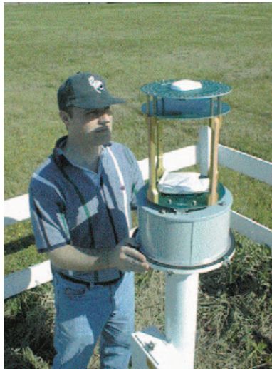
FIG. 10. The IMPACT sensor was developed by a company successor to LLP in the 1990s and replaced the original sensors that required a trailer and tower (see Fig. 4) to hold the magnetic field crossed-loop antenna.
