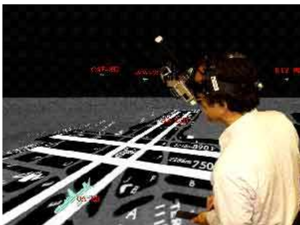
Figure 3: Virtual Tower research with Head Mounted Stereo Display. Latency Effects [Ellis et.al., NASA-Ames, Human Factors Lab.]
