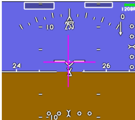
Figure 28. Baseline approach and departure dual cue (pitch and roll command bars) flight director symbology.
