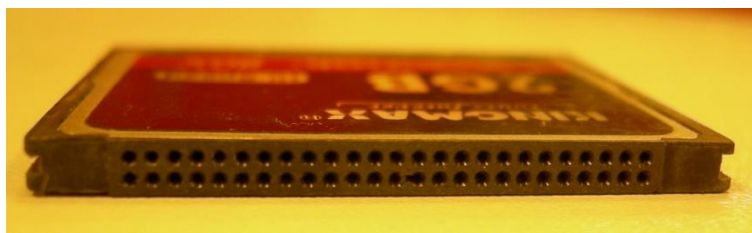
Figure 11. Memory card connector
