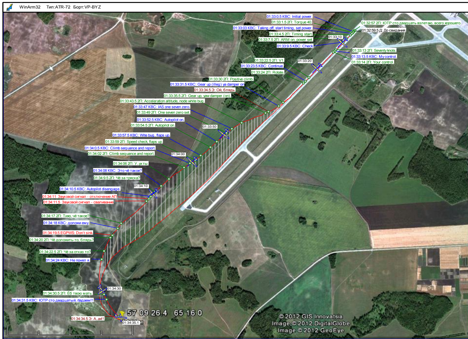
Figure 51. Flight trajectory and crew communications synchronized
