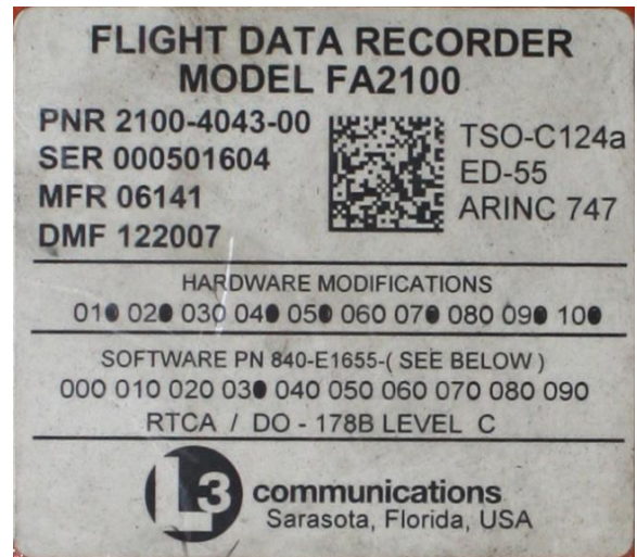
Figure 8. FDR identification label
