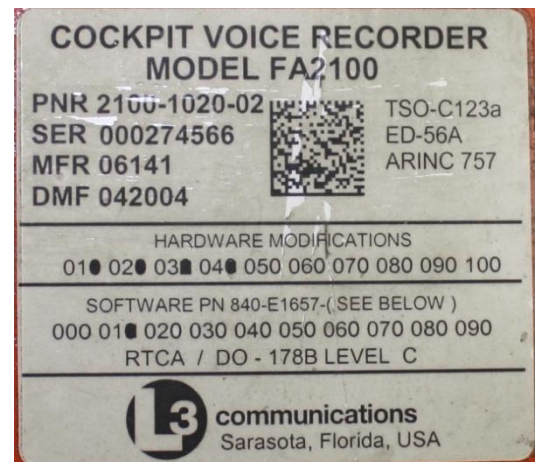
Figure 6. CVR identification label
