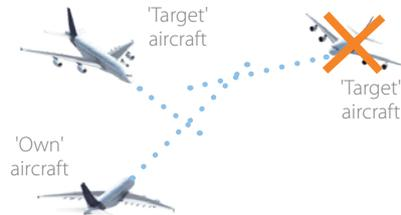
TCAS on-board the 'own' aircraft filters out the further 'target' aircraft
