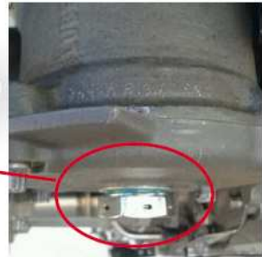
Finding: Oil filter drain plug loose
