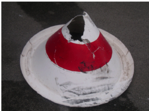
Figure 1: Damaged cone-shaped boundary marker
