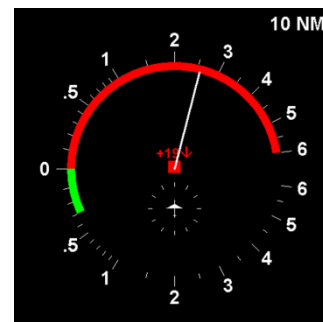
Figure 3: Initial Level Off RA as shown on a generic IVSI display (incorporating a traffic display).
