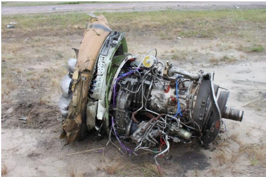
One of the engines separated from the fuselage
