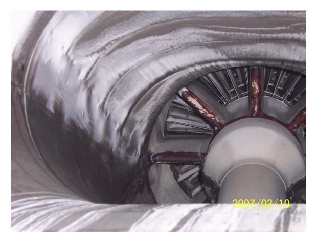
View of #2 engine intake from 10 February, 2007. Note white buildup not only on walls of intake, but also on 1<sup>st</sup> stage compressor stator and rotor blades.
