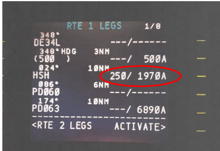
Figure 1. Picture reconstruction (for illustration purpose) showing the programmed speed/altitude constraint of “250/1970A” on SID HSN 22X
