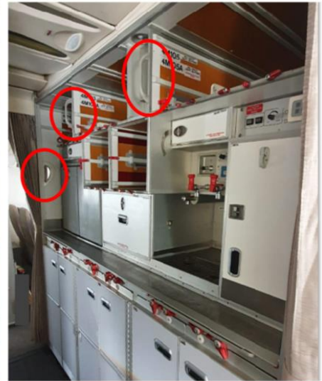
Typical galley installation with location of handholds
