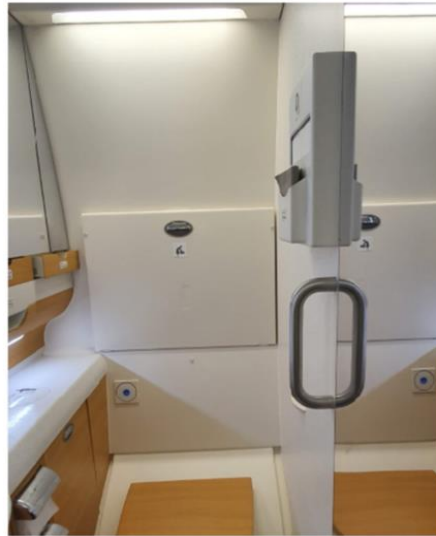
Lavatory with a single handhold
