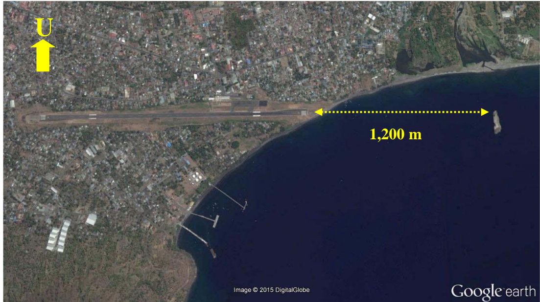
Figure 4: Atoll on final path Runway 27
