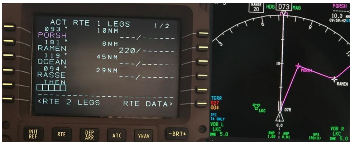
Figure 6: Simulated modified RASSE 1E SID that displayed on the CDU and ND
