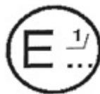
FIGURE 4. EXAMPLE OF THE REQUIRED LABELING FOR A CRS MANUFACTURED UNDER UNITED NATIONS (UN) STANDARDS
