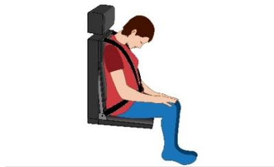
**NOTE: Figure 3 is applicable is applicable to forward-, side-, or oblique-facing passenger seats with shoulder harness.**
