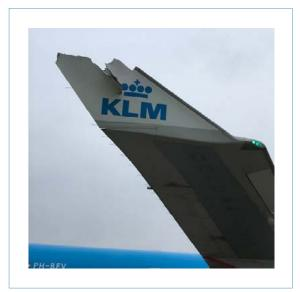
Figure 3b: Damage to the B747's right wingtip. (Source: Amsterdam Airport Schiphol)
