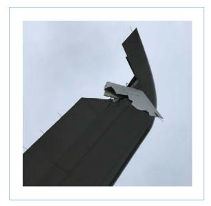
Figure 3a: Damage to the B787's right horizontal stabiliser. (Source: Amsterdam Airport Schiphol)
