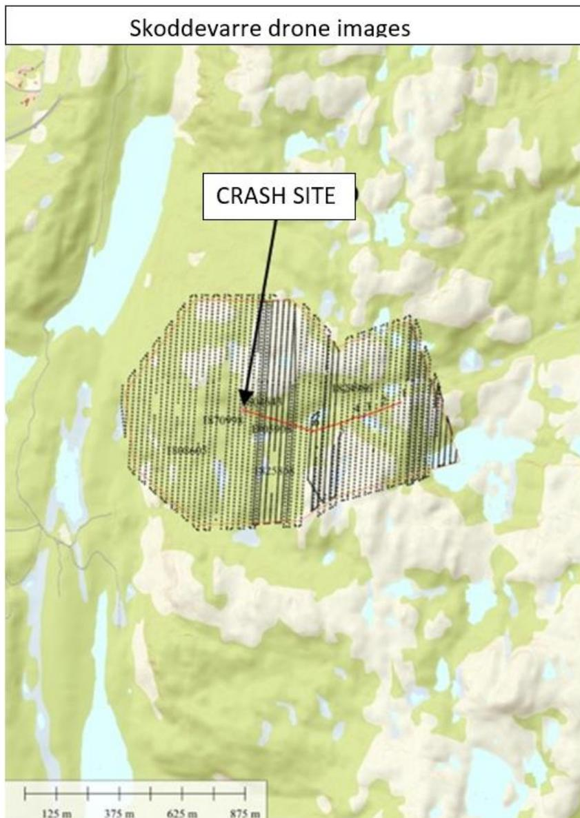
Figure 31: The red line marks the final part of the flight path. The black dots represent the 3,922 photo shots. Illustration: Geonord AS/NSIA
