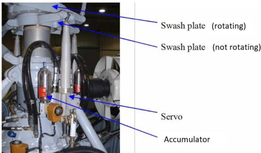
Figure 17: Rotor mast with hydraulic servos, accumulator and swashplate assembly. Photo: NSIA
