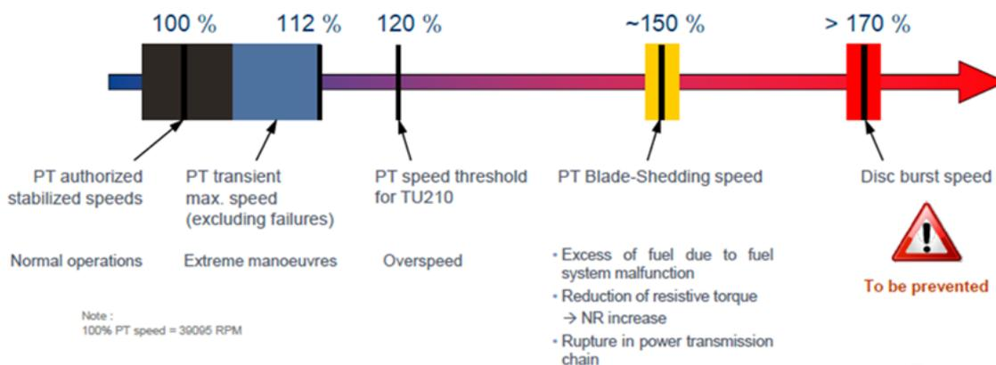
Figure 11: Rotational speed thresholds for N2 in SHE's Arriel 2D engines. Illustration: Safran Helicopter Engines/NSIA
