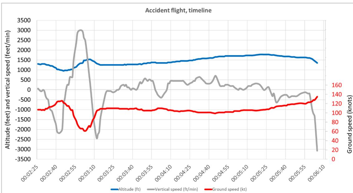
Figure 42: Flight path of the accident flight, with reference to the flight timeline. The blue curve represents altitude and the grey curve vertical speed, with the values shown on the left axis. The red curve represents ground speed, with the values shown on the right axis. Source: NSIA
