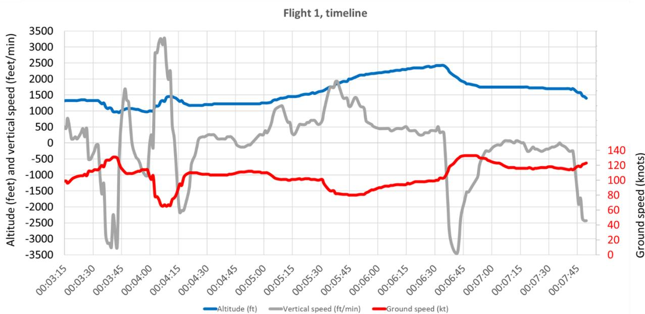
Figure 37: Flight path of first helicopter tour, with reference to flight timeline. The blue curve represents altitude and the grey curve vertical speed, with the values shown on the left axis. The red curve represents ground speed, with the values shown on the right axis. Source: NSIA
