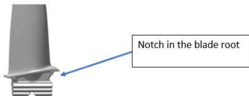
Figure 12: The arrow shows the notch at the root of the turbine blades, which is constructed to break if the rotational speed exceeds 150%. Illustration: Safran Helicopter Engines/NSIA
