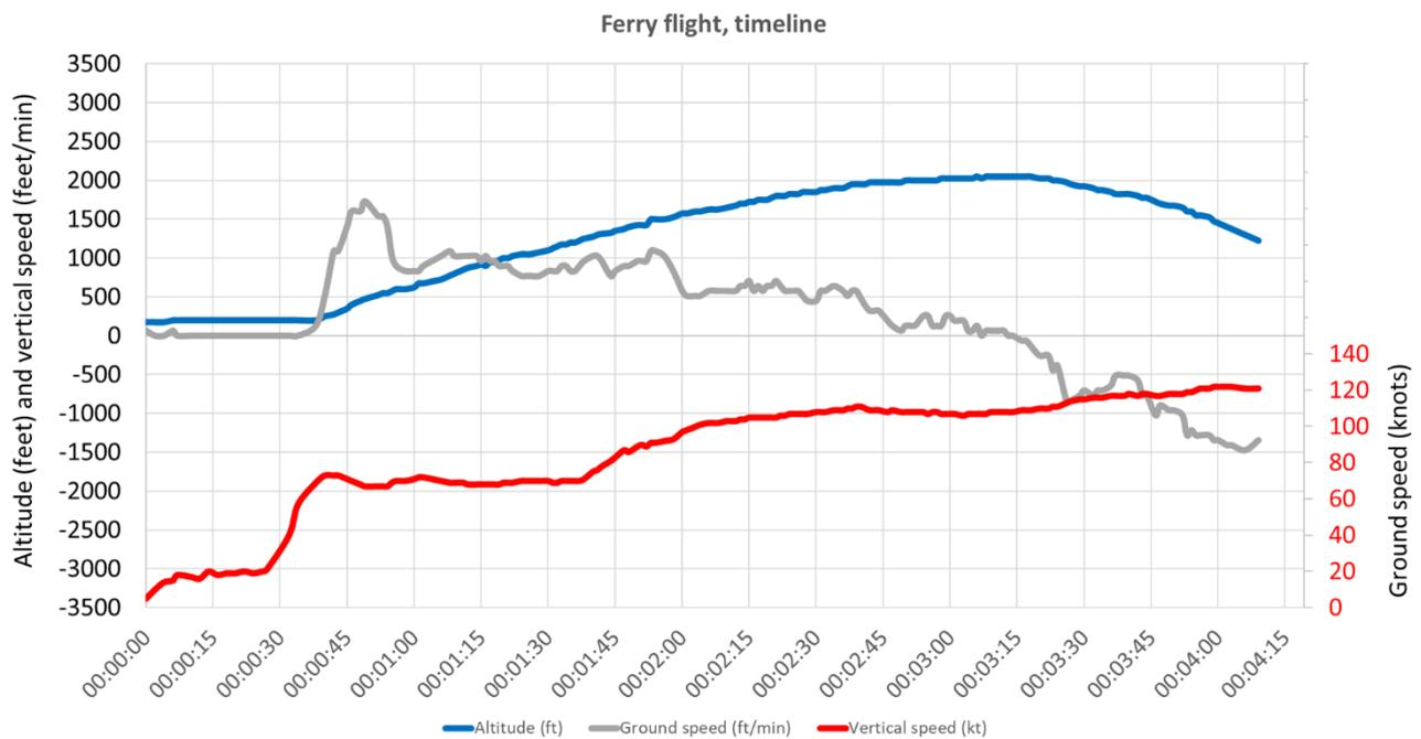
Figure 36: Flight path of parts of the ferry flight to the festival area, with reference to the timeline for the flight. The blue curve represents altitude and the grey curve vertical speed<sup>22</sup>, with the values shown on the left axis. The red curve represents ground speed, with the values shown on the right axis. Source: NSIA
