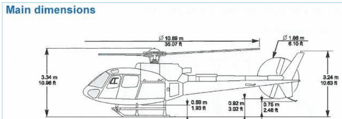
Figure 7: The main dimensions of helicopter type AS 350 B3. Drawing: Airbus Helicopters/NSIA
