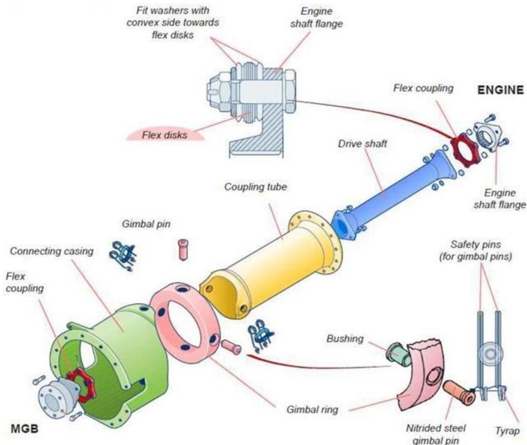
Figure 15: On the drawing, the drive shaft for the main gearbox is marked in blue and the flexible couplings at either end are marked in red. Illustration: Airbus Helicopters/NSIA
