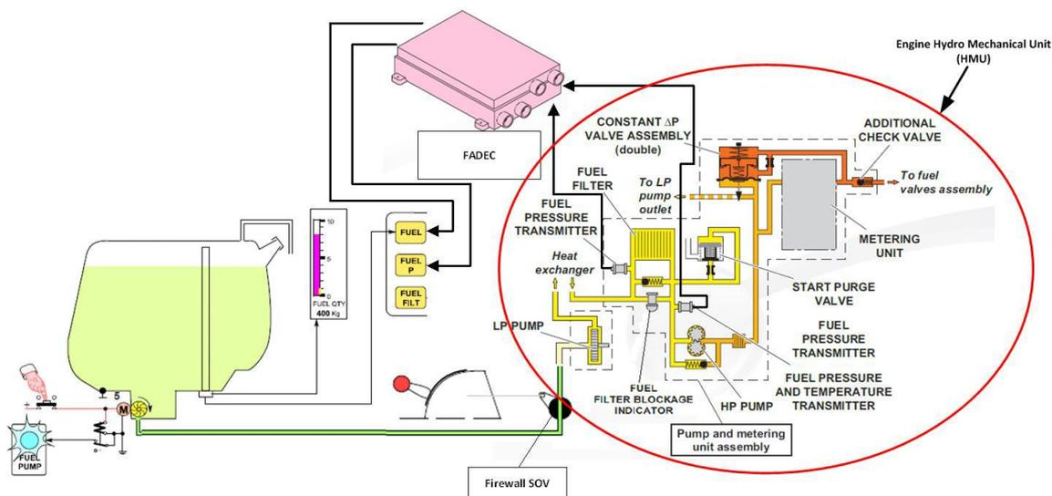
Figure 10: Simplified overview of the most important components of the helicopter's fuel system. Illustration: Airbus Helicopters/Safran Helicopter Engines/NSIA
