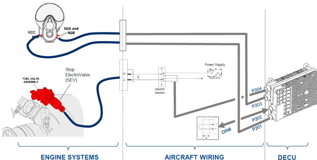
Figure 13: Schematic drawing showing the position of the N2 sensors in the engine system, as well as the fuel valve, the SEV and digital engine control unit (DECU). Illustration: Safran Helicopter Engines/NSIA
