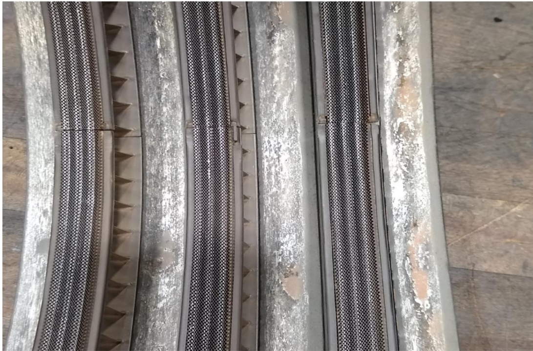
Figure 25: High pressure Compressor (HPC) blades rear cases heavy rub
