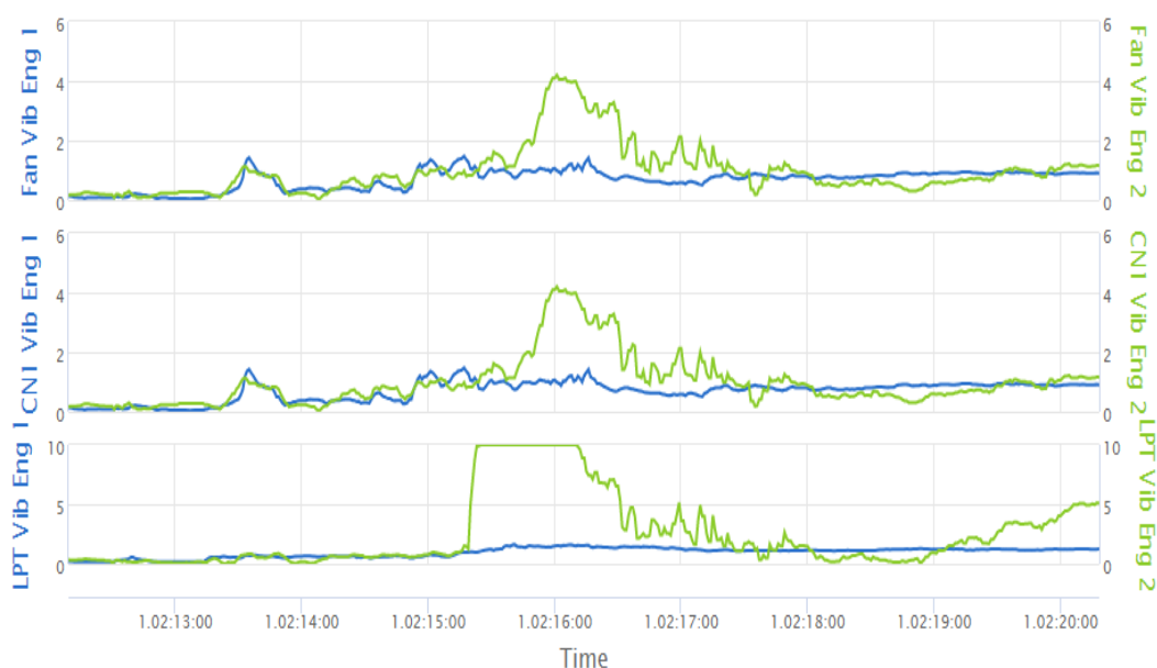
Figure 9: Engine 2 fan, compressor and turbine vibration.
