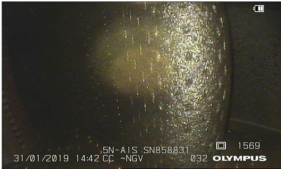
Figure 16: Nozzle Guide Vanes Leading edge and Preservation Oil
