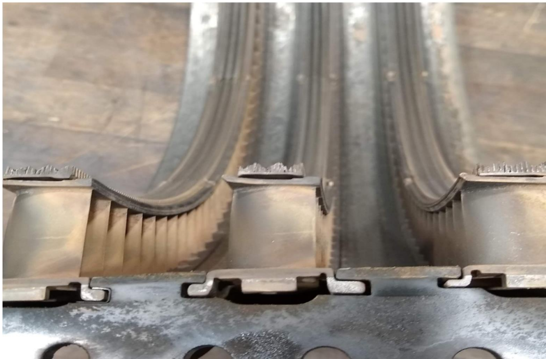
Figure 26: High pressure Compressor (HPC) blades rear cases rub
