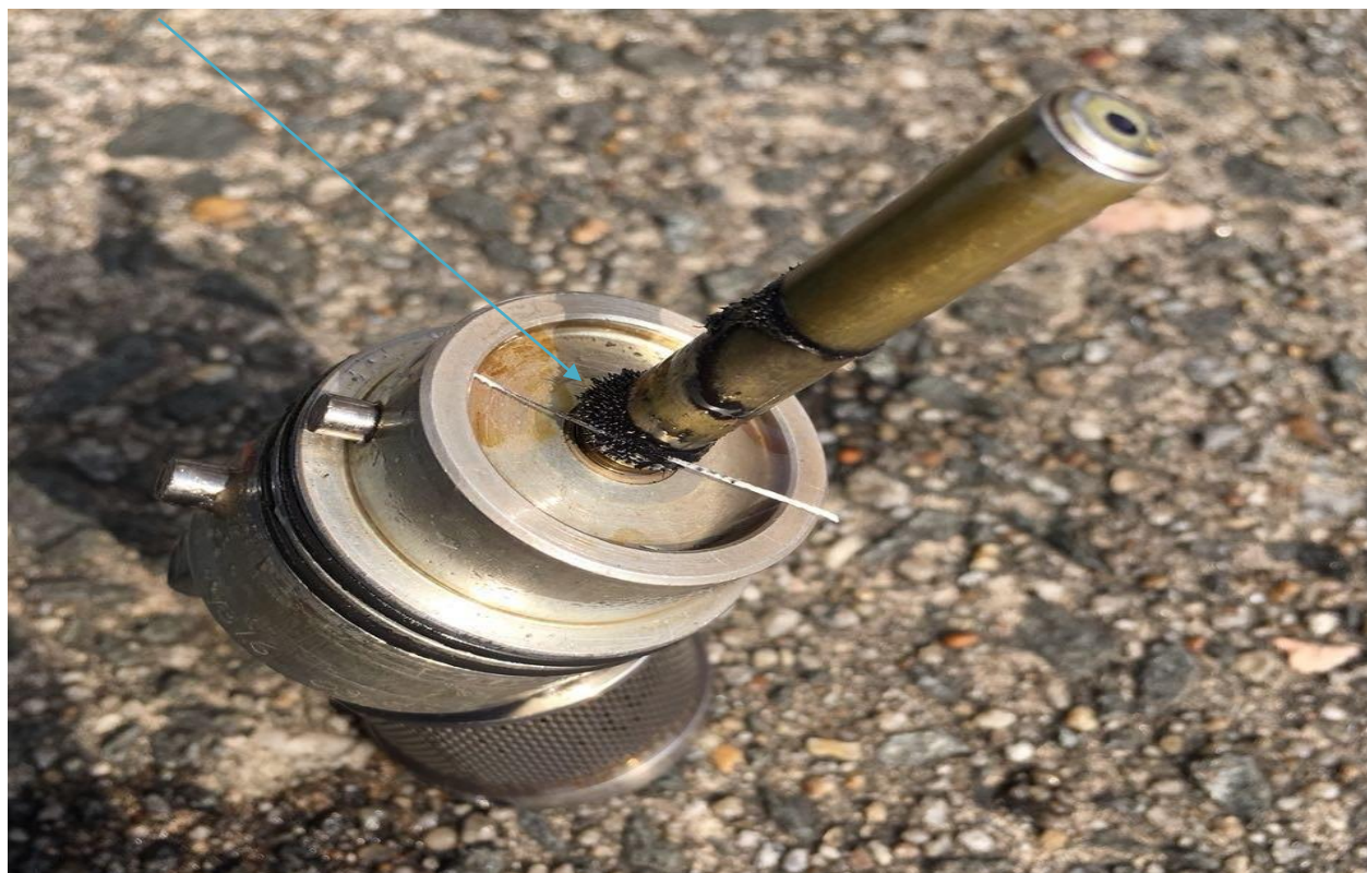
Figure 19: Number two engine Magnetic Chip Detector aft sump showing metallic particles
