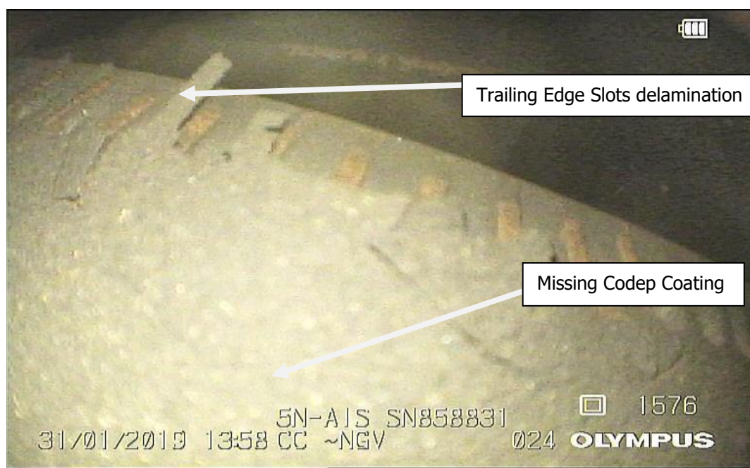
Figure 15: Trailing edge slots delamination and missing codep coating of HPT blade
