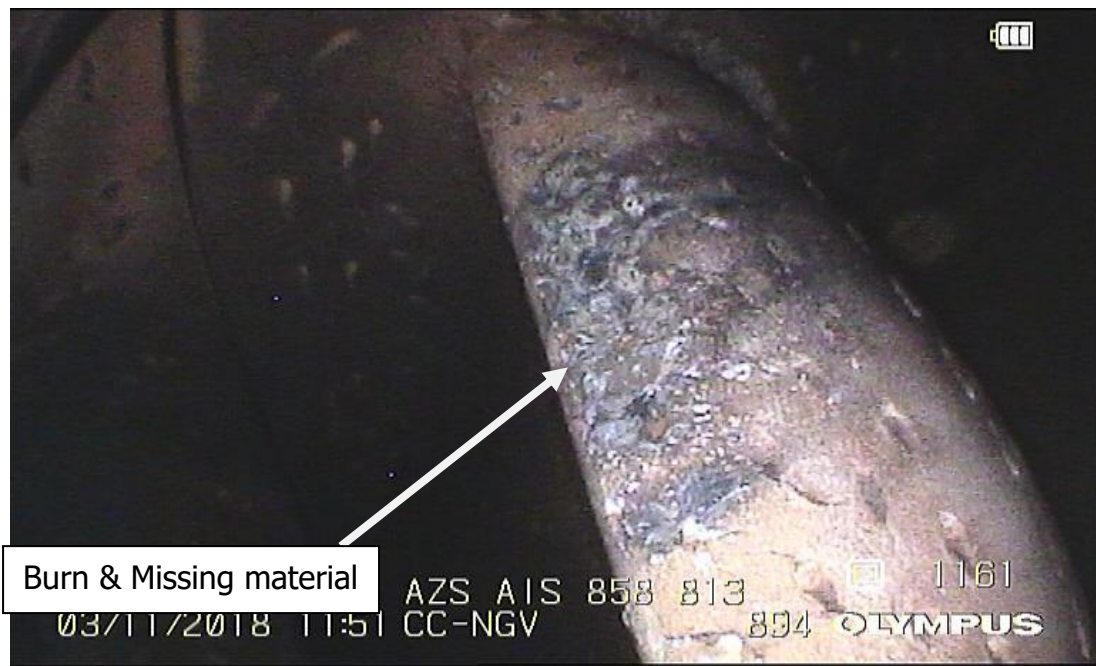
Figure 14: Burn and missing material of the HPT nozzle
