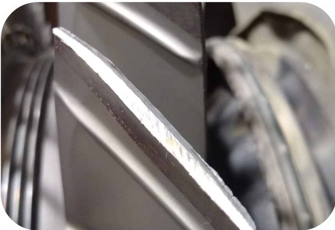
Figure 21: High Pressure Compressor Blades tip rub
