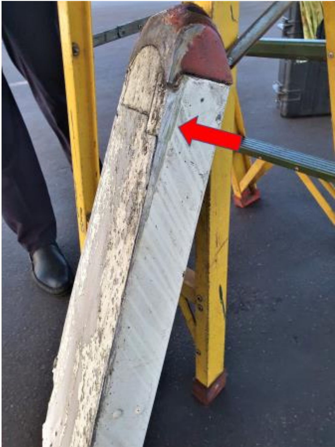
Figure 4: Torn-off tailskid plate with fresh scrape marks.
