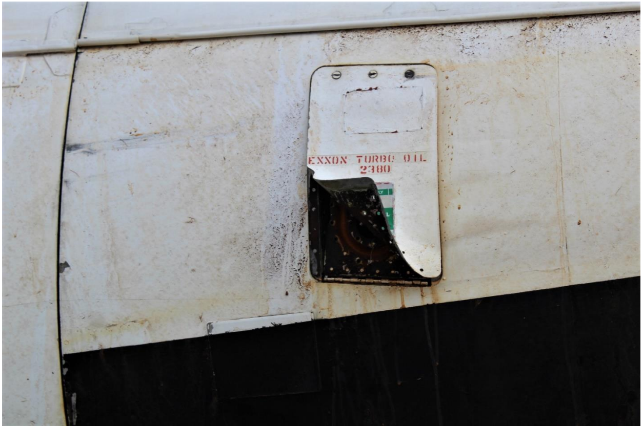
Figure 6: Damage to no. 2 engine oil servicing panel.
