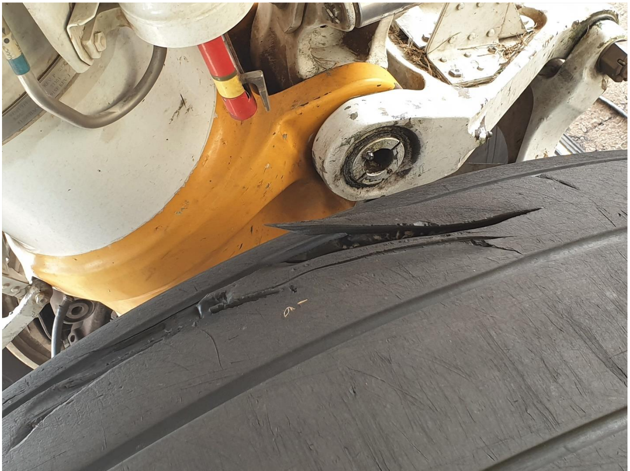
Figure 3: Tire damage as a result of impact with runway edge lights.
