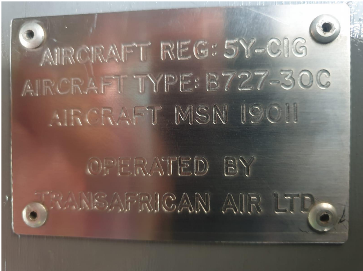
Figure 11: Identification plate showing Kenyan registration.
