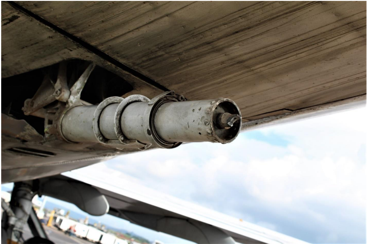
Figure 5: Broken tailskid cylinder pointing rearward.
