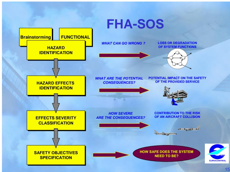
Figure 3.1: Safety Objective Specification (without “assess intended aggregated risk”)
