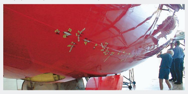
lightning strike is damage caused to bonding straps. These straps can become crushed during a lightning strike due to the high electromagnetic forces.
