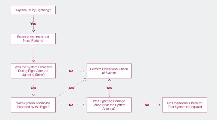
found in the structural repair manual (SRM) for each airplane model. Maintenance personnel should restore the original structural integrity, ultimate load strength, protective finish, and materials after a lightning strike.
