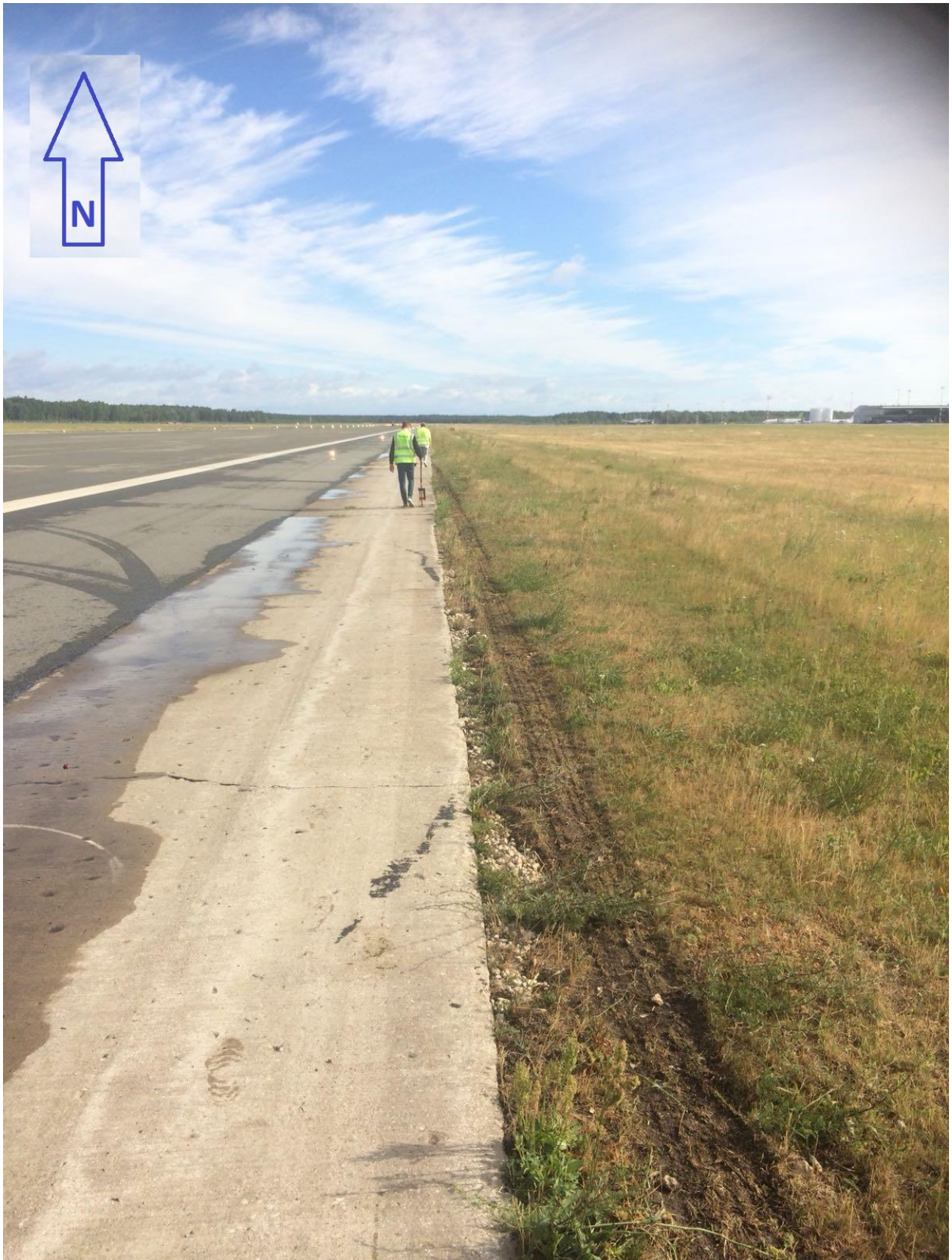
Picture 2 Length of the of the aircraft's MLG left outer tire trace in the grass 121m
