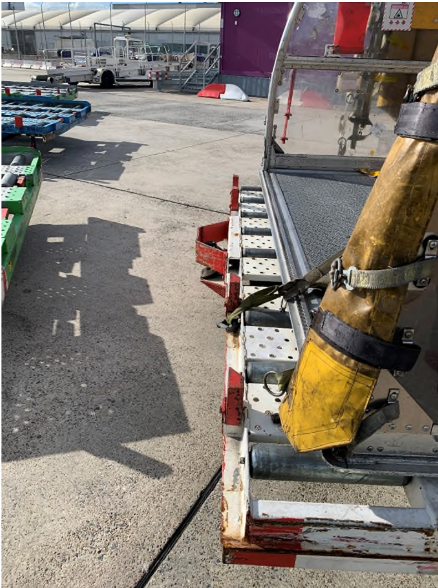
Fig. 7: Example of a pallet car with open safety locks
