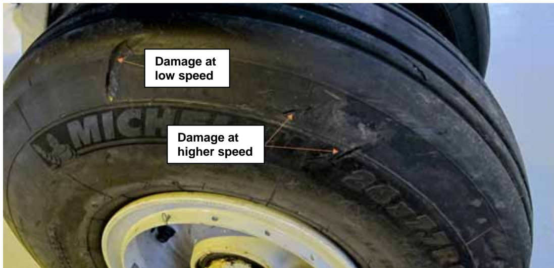
Figure 4. Damage to the nose gear tyre.
