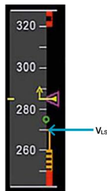
(fig.3) V<sub>LS</sub> on the PFD speed scale
