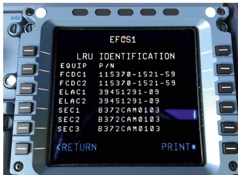
“ Operational software identification (LRU IDENTIFICATION) is the ultimate safety barrier to prevent inappropriate FLS and aircraft configurations. ”
