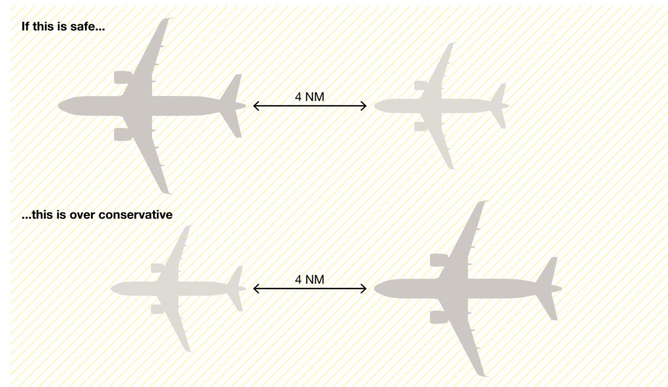
**RECAT 1 FAA:** The FAA decided to reclassify the aircraft by MTOW and wingspan. The RECAT FAA is implemented on several US airports.
