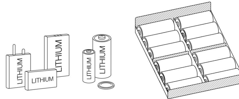
(fig.3) Types of Lithium batteries: single/multi cells
