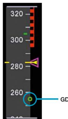
(fig.1) GD on the PFD speed scale
