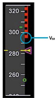
(fig.4) V<sub>MO/M<sub>MO</sub></sub> on the PFD speed scale
