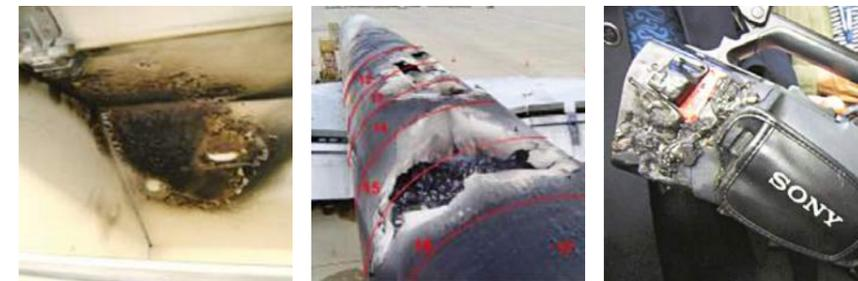
Damage to cabin overhead compartment video camera
