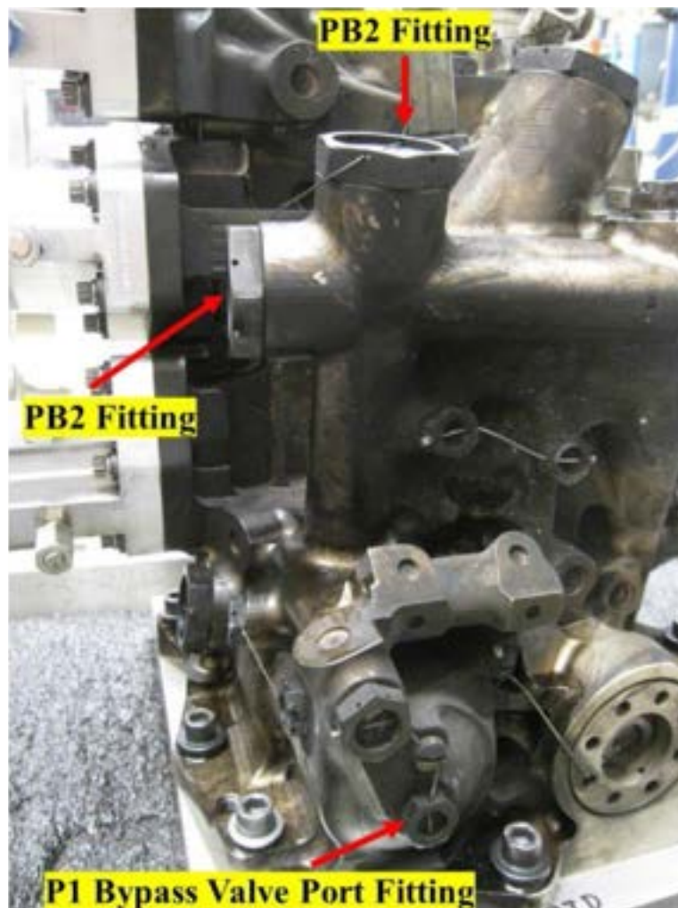
Figure 36: Nitrogen Leak Locations
