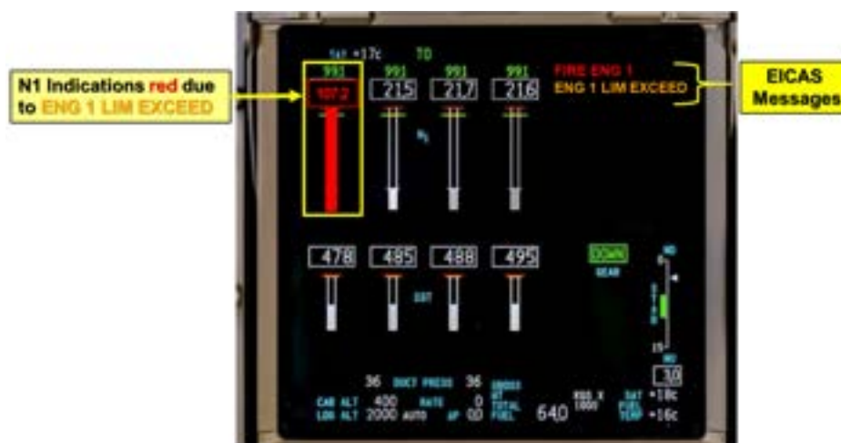
Figure 1: Example of Displayed EICAS Indications and Messages
