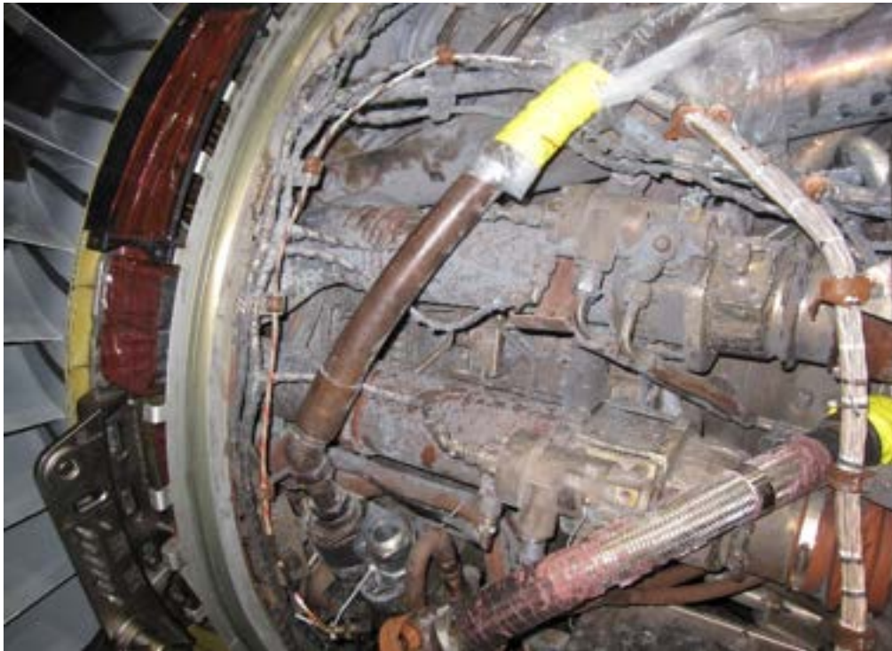
Figure 15: Left Side Close-Up of Thermal and Fire Damage
