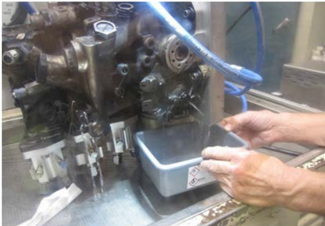
Figure 39: Calibration Fluid Collected From P1 Bypass Valve Port Fitting
