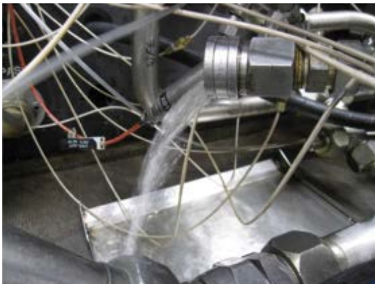
Figure 51: Fluid Leak from P1 Bypass Valve Port Fitting
