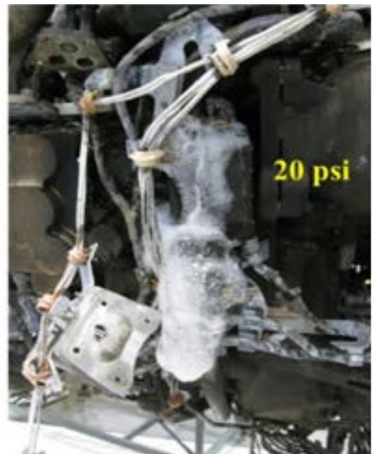
Figure 26: Leaking from Top and Bottom of FFT
