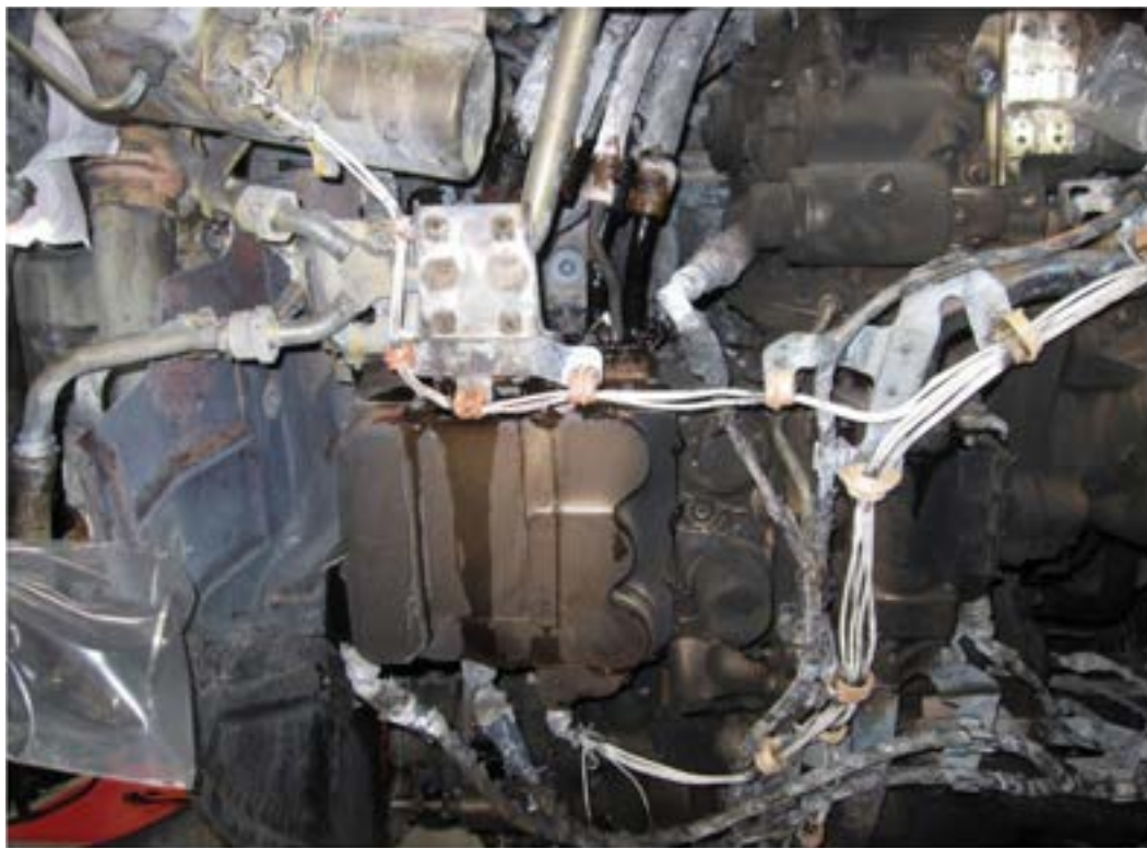
Figure 23: Fuel Leaking from Multiple Locations of FMU
