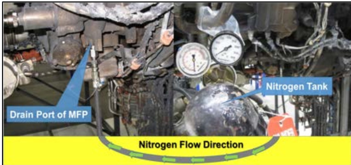
Figure 22: Leak Check Set-Up
