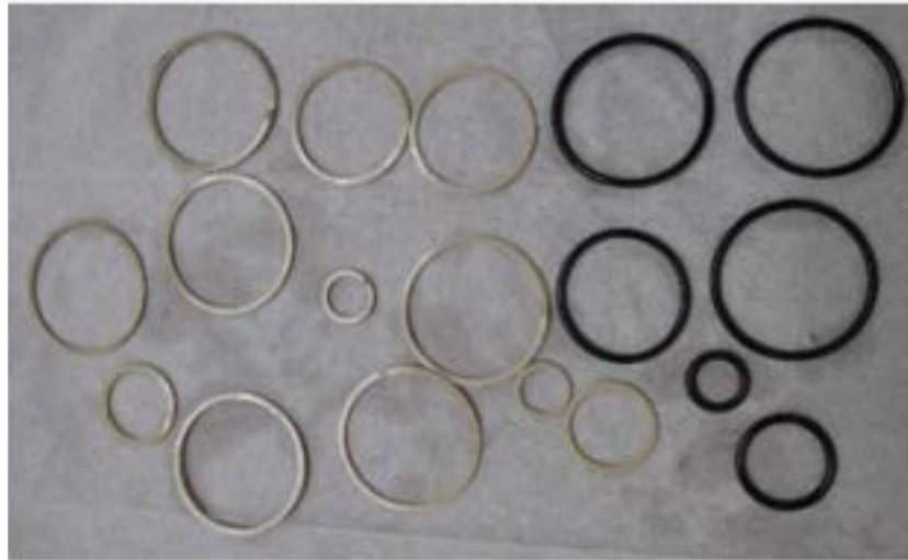
Figure 31: Condition of Packing & Back-up Split Rings
