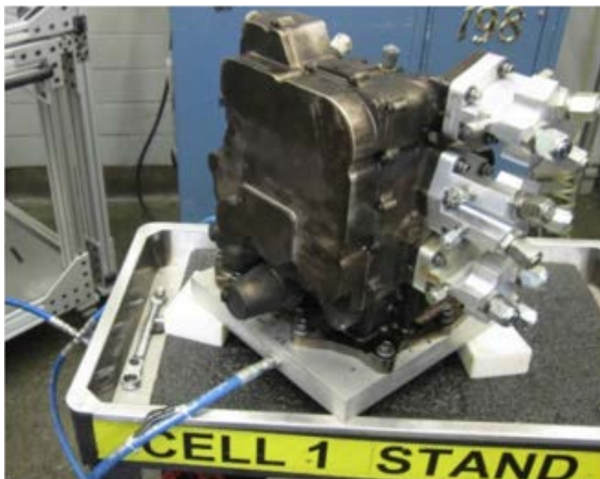
Figure 35: Nitrogen Test Set-up
