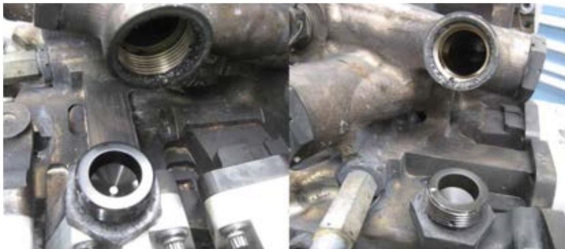
Figure 42: PB2 Bypass Packings Consumed
