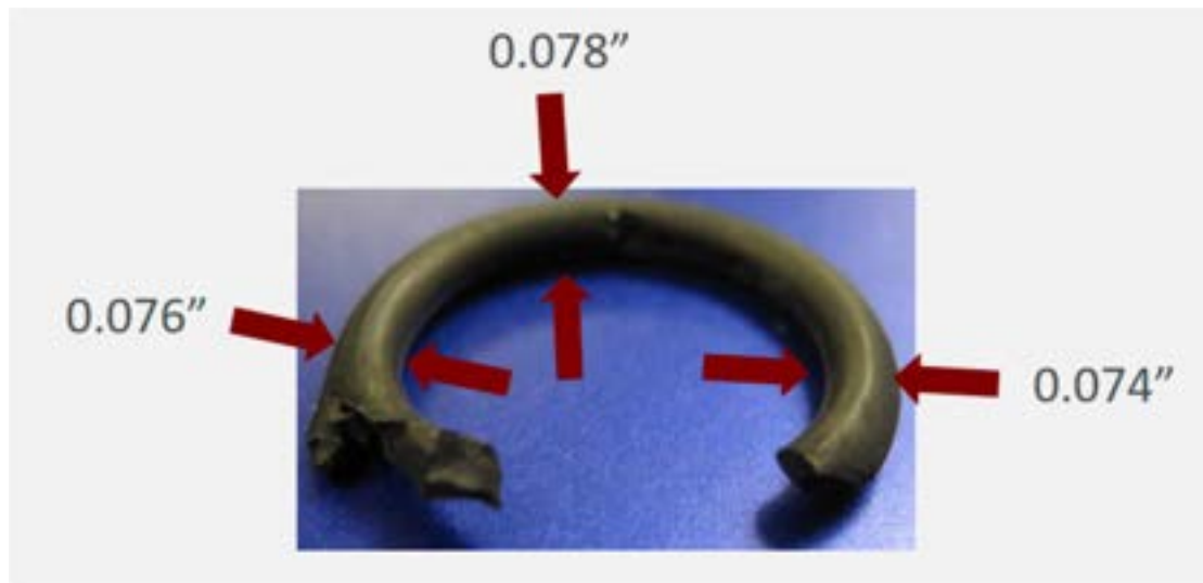
Figure 43: Damaged P1 Bypass Valve Port Fitting Packing
