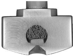
Figure 13. terminal (J) CT scan
