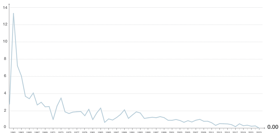
Yearly hull loss accident rate per million flights
