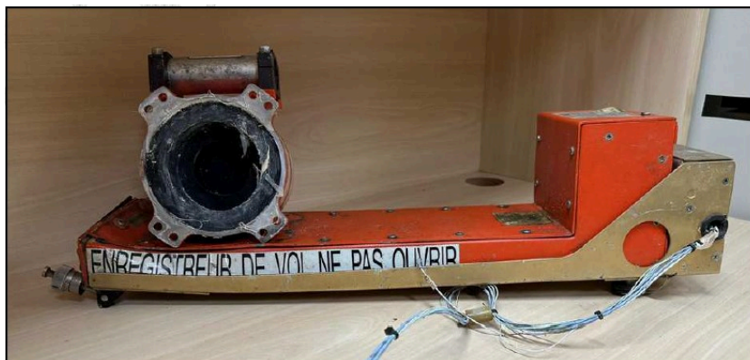
Figure 29 - Flight Data Recorder installed in the PS-VPB.
