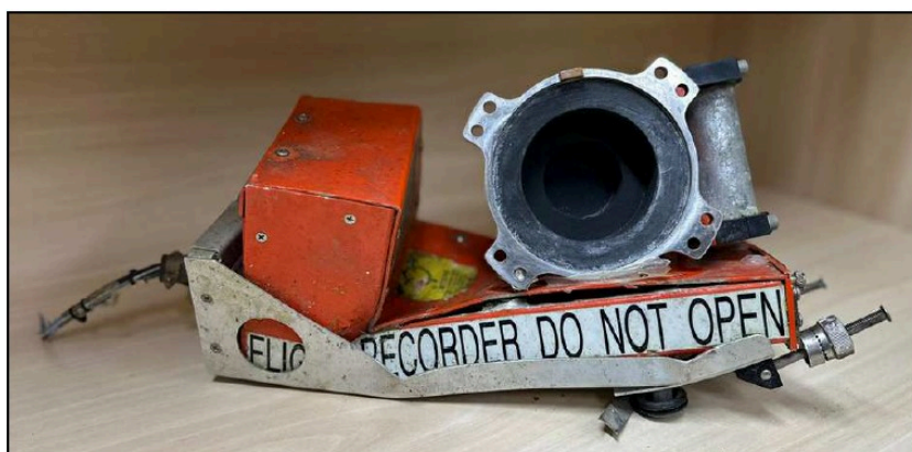
Figure 30 - Cockpit Voice Recorder installed in the PS-VPB.
