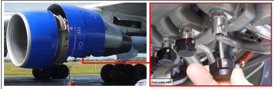
Figure No. 1: Location of MCDs at the base of the engine (typical installation)
