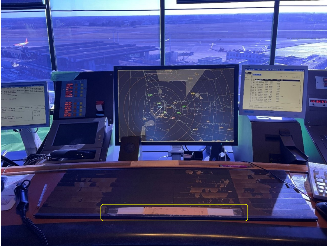
Figure 15: photo of the strip board used on the day of the serious incident; theoretical positioning of a strip for an aeroplane at the runway threshold, represented by a white band, here covered with transparent adhesive tape.
