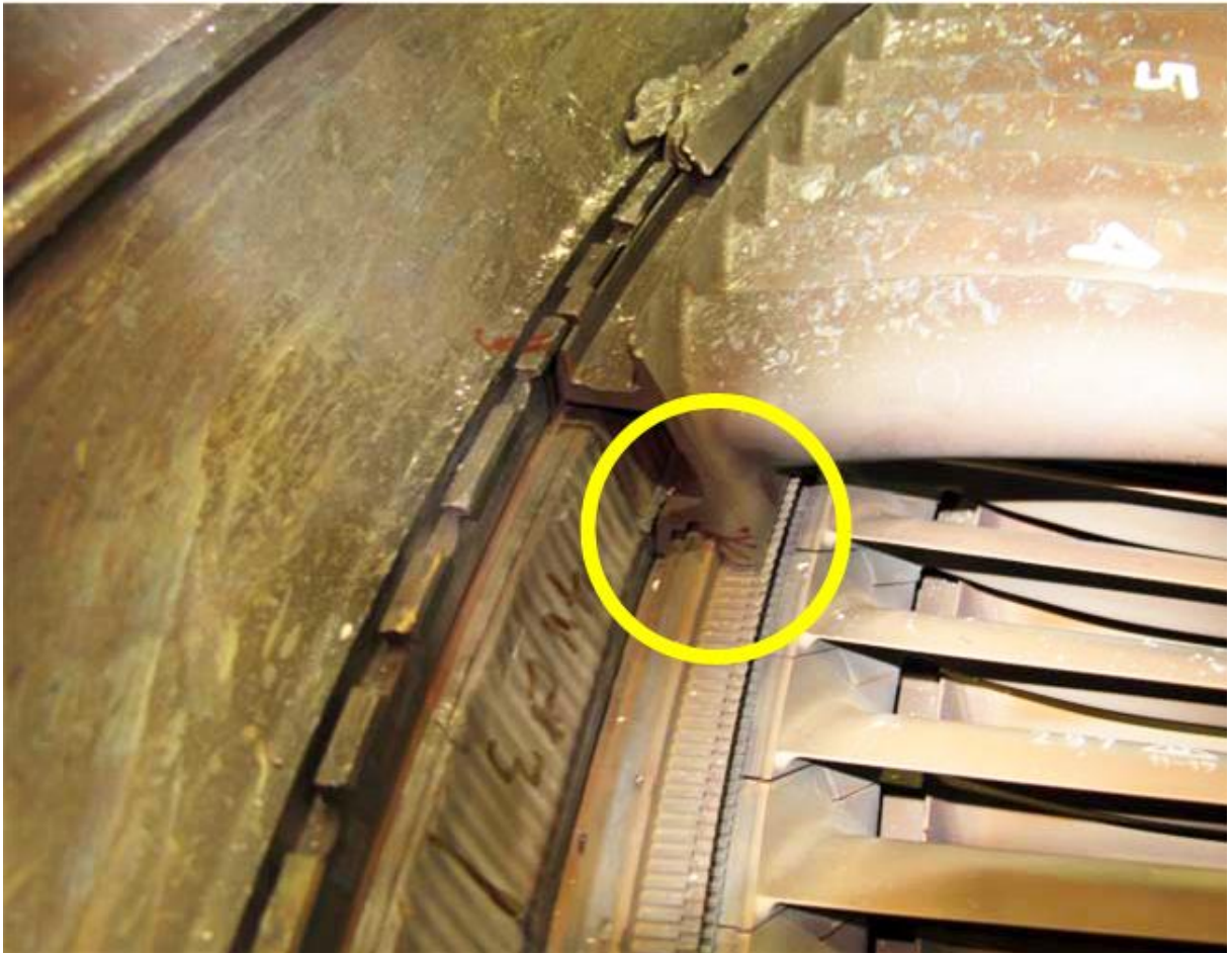
Fig. 23: Vane Cluster # 4, principle drawing and close up, yellow circle shows an outside diameter gusset
