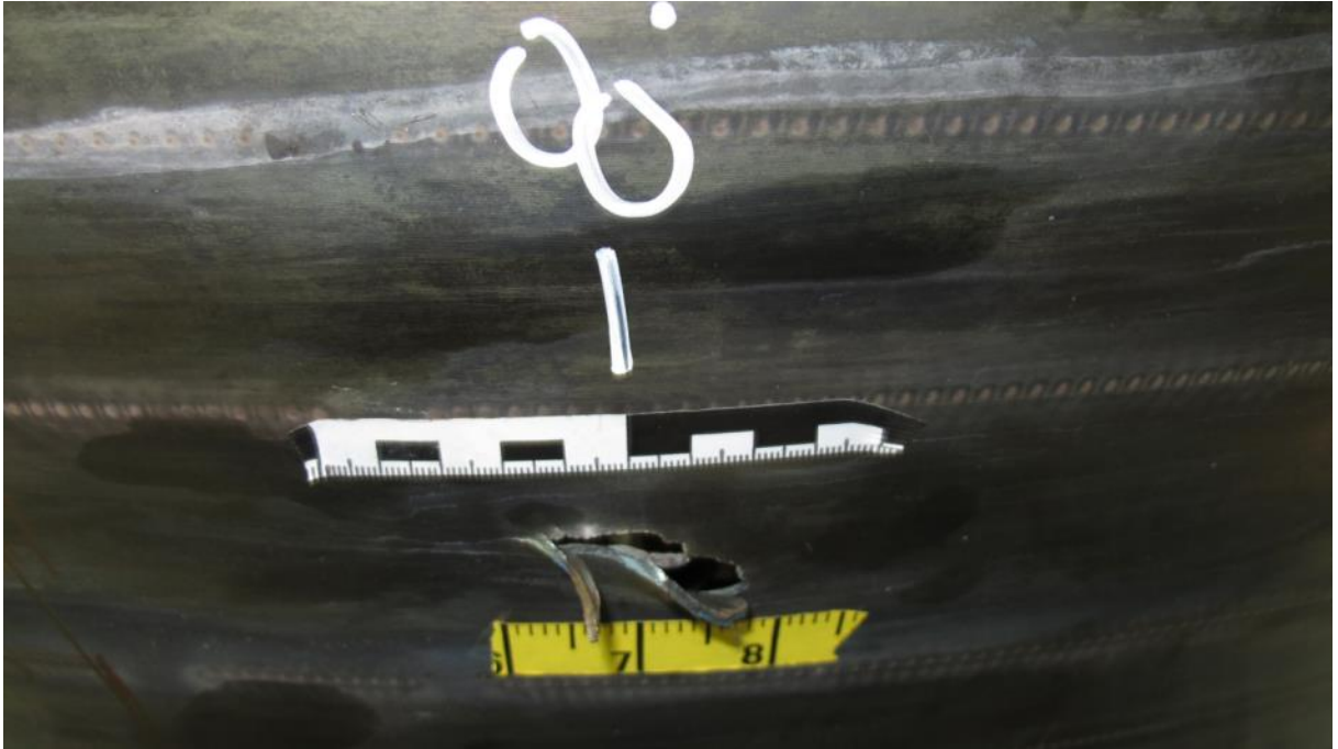
Fig. 38: Damaged LPT housing at 0830 position (footnote 19)
