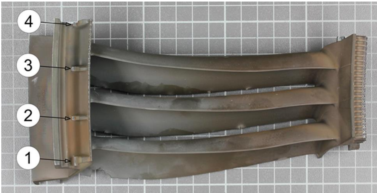
Fig. 24: Vane cluster No. 4 including numbering of the gussets
