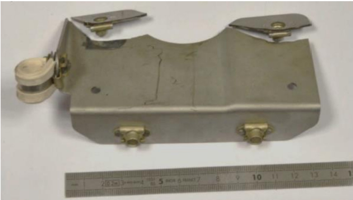
Fig. 43: Fatigue fracture at the Hydraulic Line Bracket F29030080, in detail
