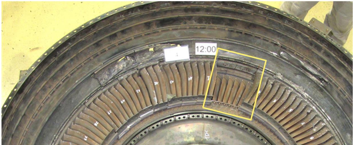
Fig. 21: View of the 4 th guide vane stage. The yellow marking shows the position of the two missing vane cluster
