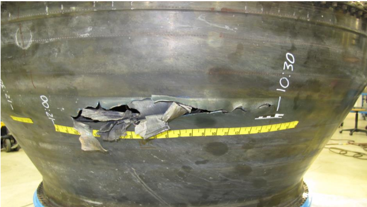
Fig. 36: Damaged LPT housing, white markings mark the position circumference (footnote 19)
